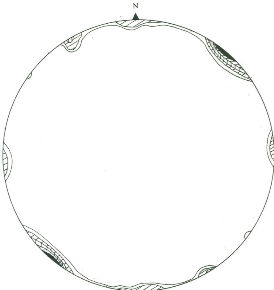
Fig. 7—Stereogram of joint-planes in the Ndeyini area; 92 measurements, contours at 5, 10, 20, 30 and 35 per cent per one per cent area.
